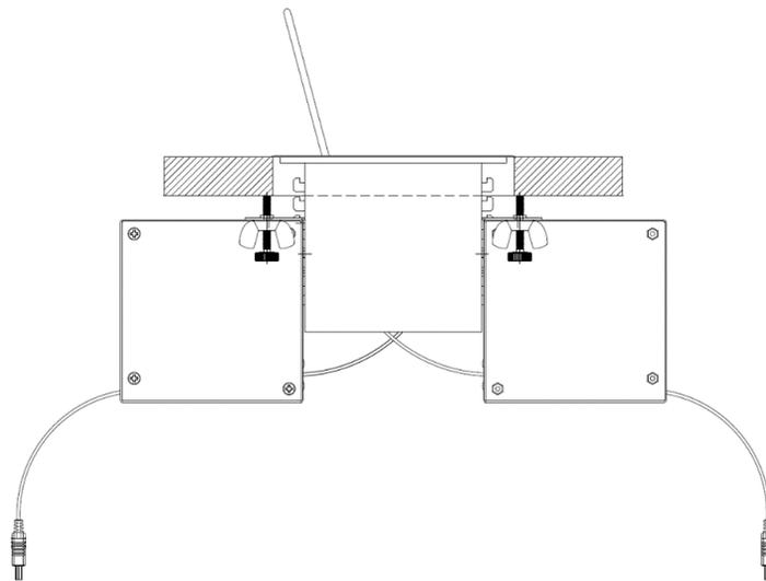
Diagram 5: Mounted on a CNK200 Side View
